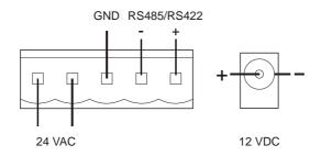
IMPORTANT: The 24 VAC power supply must be a class 2 type. Do not make any connection to ground.
