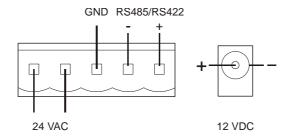
IMPORTANT: The 24 VAC power supply must be a class 2 type. Do not make any connection to ground.
