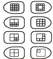
The Live and Playback images in a multiscreen display may be transposed by pressing the **Multiscreen** button that corresponds with the current multiscreen display (e.g., If the current display is a 13-way multiscreen with the centre cameo being a playback image and the rest of the cameos being live images, pressing the **13-Way Multiscreen** button will result in the centre cameo being live and the rest of the cameos being playback images).
