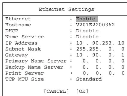
If **Ethernet** is enabled but **DHCP** and **Name Service** are disabled, the user can set the **IP Address**, **Subnet Mask** and **Gateway** manually.
