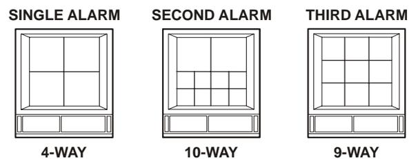
**Single Alarm:** When a single alarm is received, the unit changes to 4-way display. By default this display will contain the camera in alarm (i.e., if alarm input 3 is activated, camera number 3 will be displayed), and three associated cameras. These cameras can be defined as a group in the menu system (see **Alarm Action Setup** on page 34). The top left cameo displays the camera in alarm.
