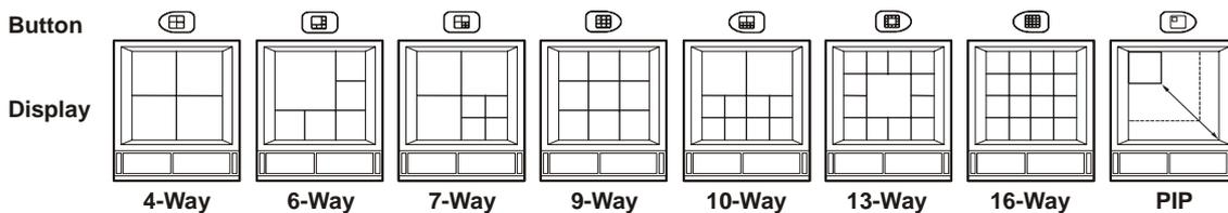
The multiscreen display is limited to the number of camera inputs on the unit.
