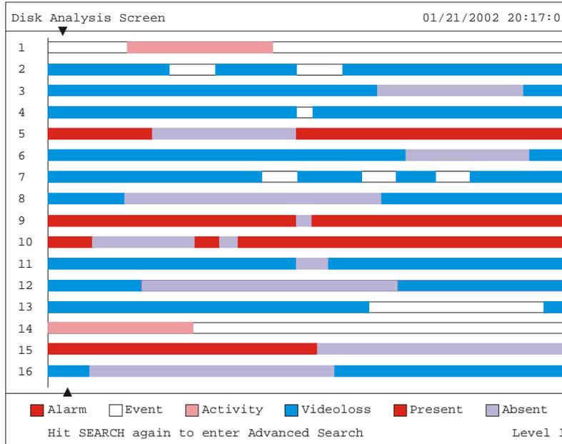
Rotating the **Jog** moves the two arrow cursors across the representation of the recorded video. As the cursors move across the screen the corresponding disk time is indicated in the upper right of the screen. The video representations are colour-coded by category. Rotating the **Shuttle** expands (zooms) the display. The lowest level (most detail) is indicated on screen with an **(L)**. Pressing the **Enter** button will start Playback from the cursor location.
