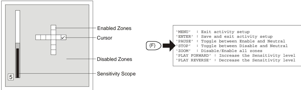
The **Stop** and **Pause** buttons are used to determine the action of the cursor, and it's current status can be seen by the way in which it is displayed. It has three possible modes NEUTRAL (blank square), ENABLE (square with a tick inside) and DISABLE (square with a cross inside). No Action will have no effect on the current cursor position; Enable will change the current cursor position to an active zone; Disable will change the current cursor position to a non-active zone.
