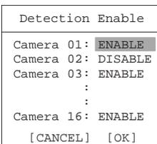
To save the changes and exit the dialog, use the **Jog** to select **[OK]**, then press the **Enter** button. To exit the dialog without making changes, use the **Jog** to select **[CANCEL]**, then press the **Enter** button.
