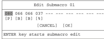
Use this dialog to create the RS232 command string. Press the **Enter** button to enter and exit the submacro edit mode. Rotate the **Shuttle** to navigate among the fields and use the **Jog** to change the values. Each byte value can be set from 0 to 255. To save the sub-macro, use the **Jog** to navigate to **[OK]** and press the **Enter** button.
