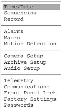
Once the required drop-down menu is opened, rotate the **Jog** to move the cursor through the items in it. A drop-down menu will look like the example on the left.
