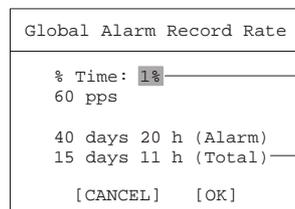
Estimate of the % of time the unit will typically spend in alarm mode. For example if you expect to have about 5 total periods of alarms each day, each lasting 3 minutes on average, then the % of the time will be 1%. (15 mins/24 hours)
