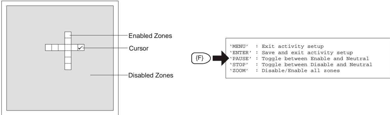
The **Stop** and **Pause** buttons are used to determine the action of the cursor, and its current status can be seen by the way it is displayed. It has three possible modes NEUTRAL (blank square), ENABLE (square with a tick inside) and DISABLE (square with a cross inside). No Action will have no effect on the current cursor position; Enable will change the current cursor position to an active search zone; Disable will change the current cursor position to a non-active search zone.
